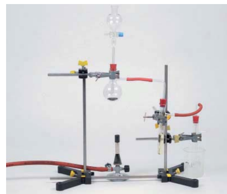
The cracking of petroleum.
