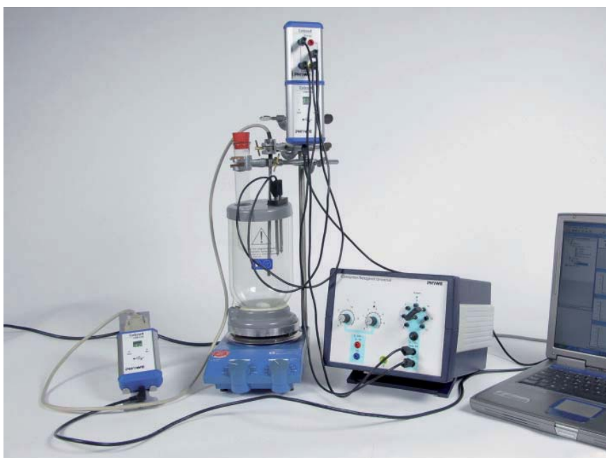
Temperature-time curve for the melting process of dioxan and determining the heat capacity of the system.
