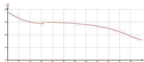
Crystallisation curve of naphthalene.
