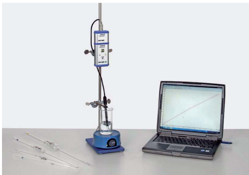
Conductivity of a strong electrolyte as a function of the concentration.
