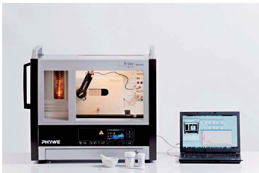
Bragg-Cu-K \alpha and Cu-K \beta lines of germanium powder
