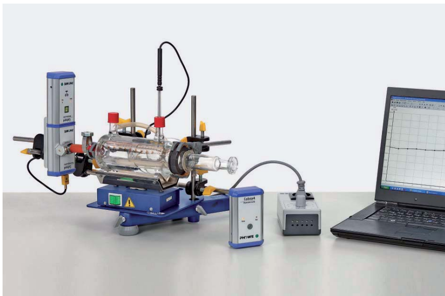
Correlation between volume and pressure under isothermal conditions.
