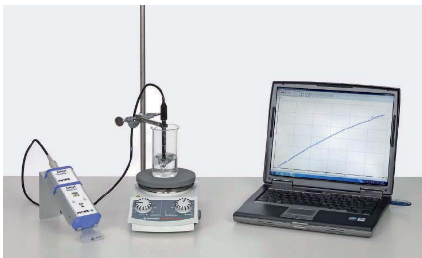
Conductivity of an aqueous potassium chloride solution at different temperatures.
