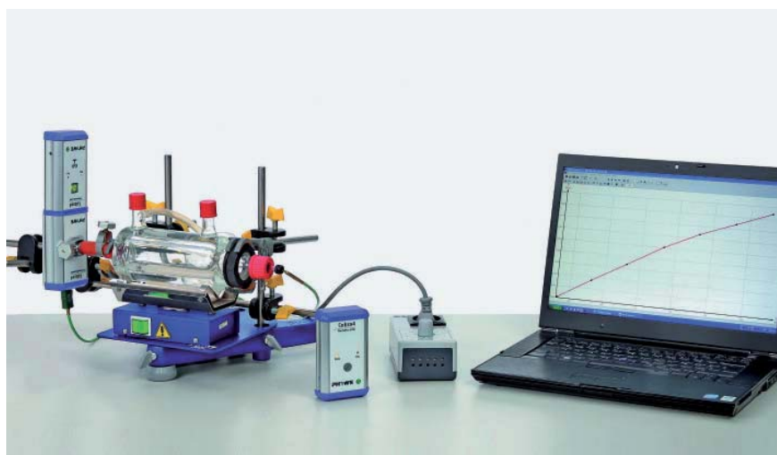
Dependence of the pressure on the temperature under isochoric conditions.
