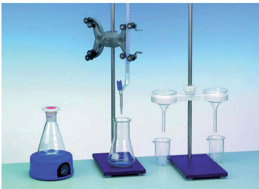
Investigation of the adsorption isotherm for the citric acid/active carbon system.
