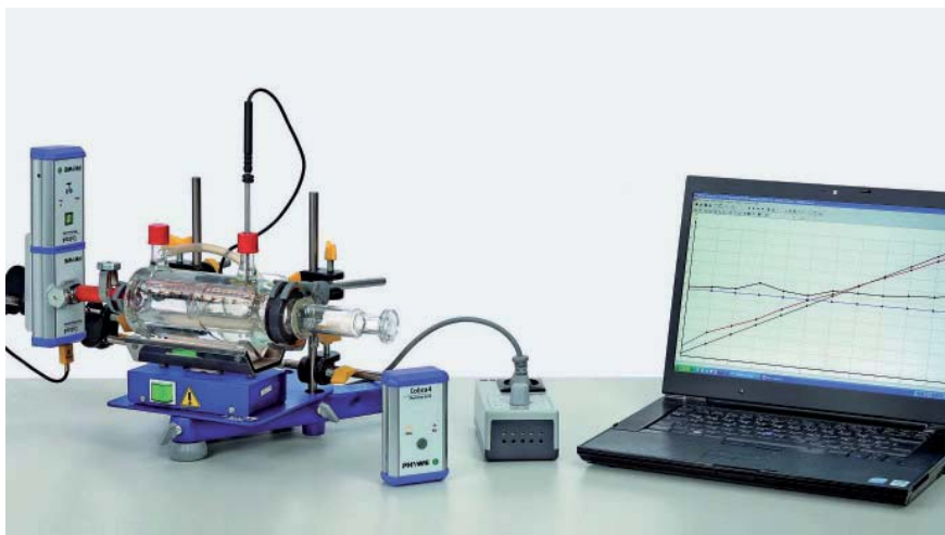
Dependence of the volume on the temperature under isobaric conditions.
