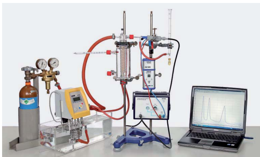
Gas chromatographic separation of a mixture of butane gases.
