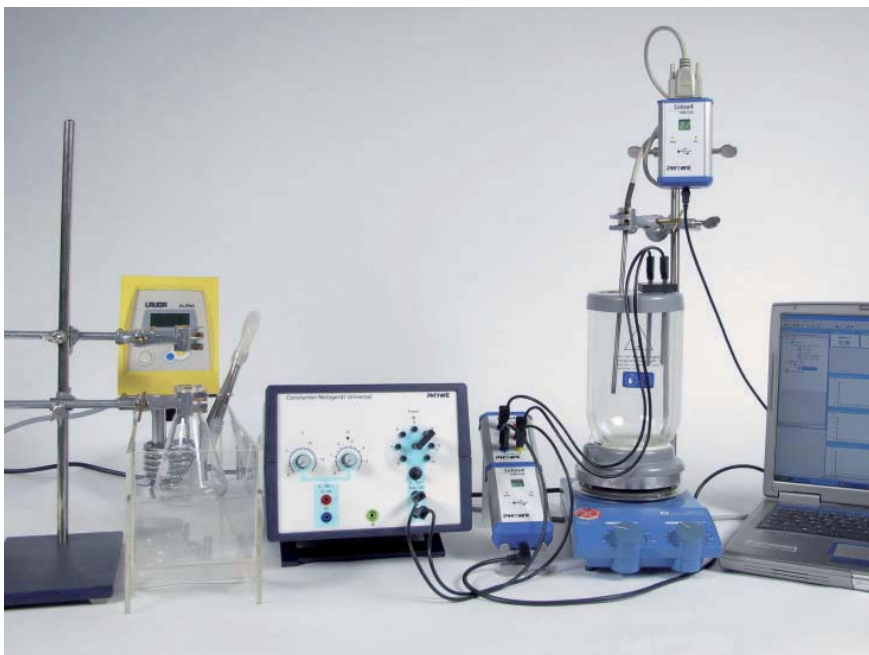
Temperature-time curve of the mixing of two miscible fluids and determining the heat capacity of the system.
