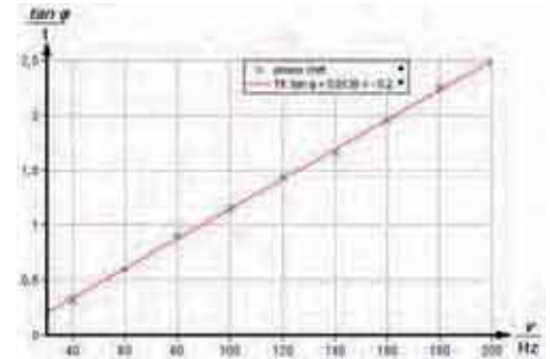
Self-inductance and resistor in series: \tan \phi as a function of v .
