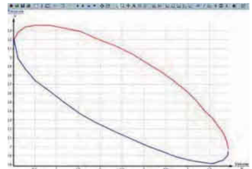
Pressure as a function of volume for the Stirling process.
