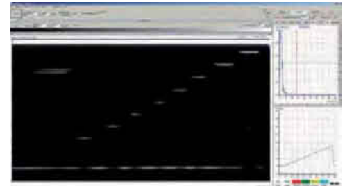
B-Scan image produced with the 2MHz probe.
