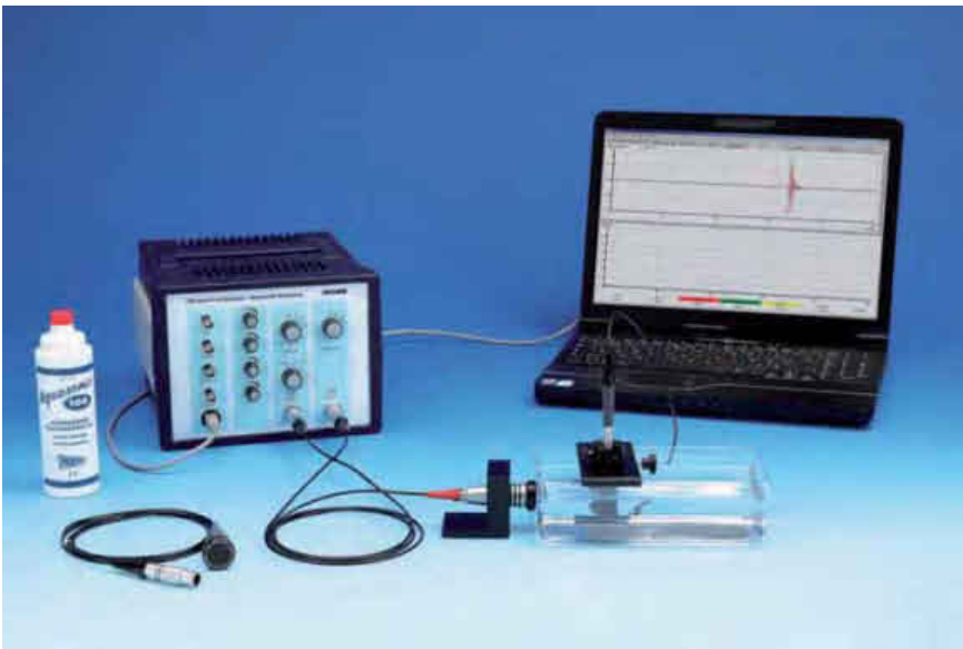
Sound field of a 2-MHz-probe with a diameter of 16 mm.
