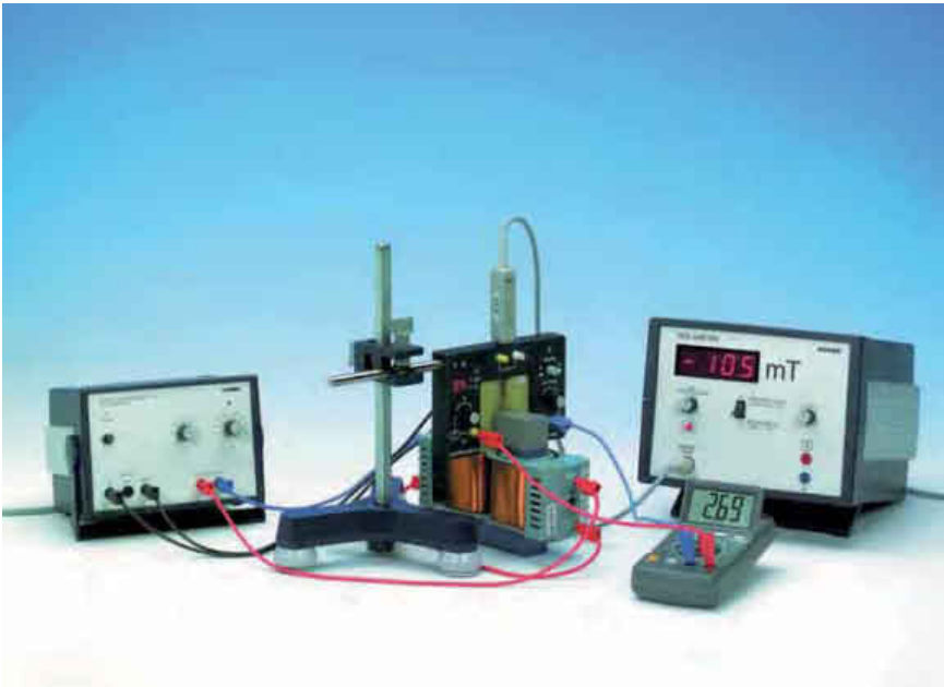
Hall voltage as a function of magnetic induction.
