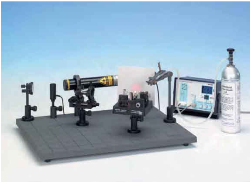
Michelson's setup for interference.
