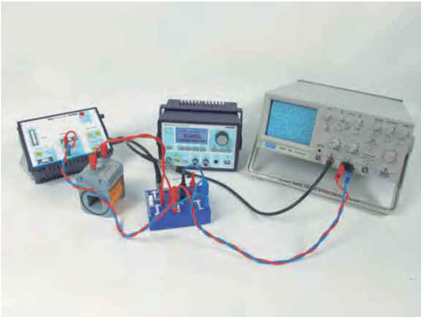
Voltage tapped off the diode at U_{ss}=9V . The circuit is oscillating chaotically.
