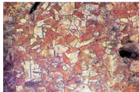
Copper, etched in sol. 5, grain contrast/precip. etching, magnification approx. 100x.
