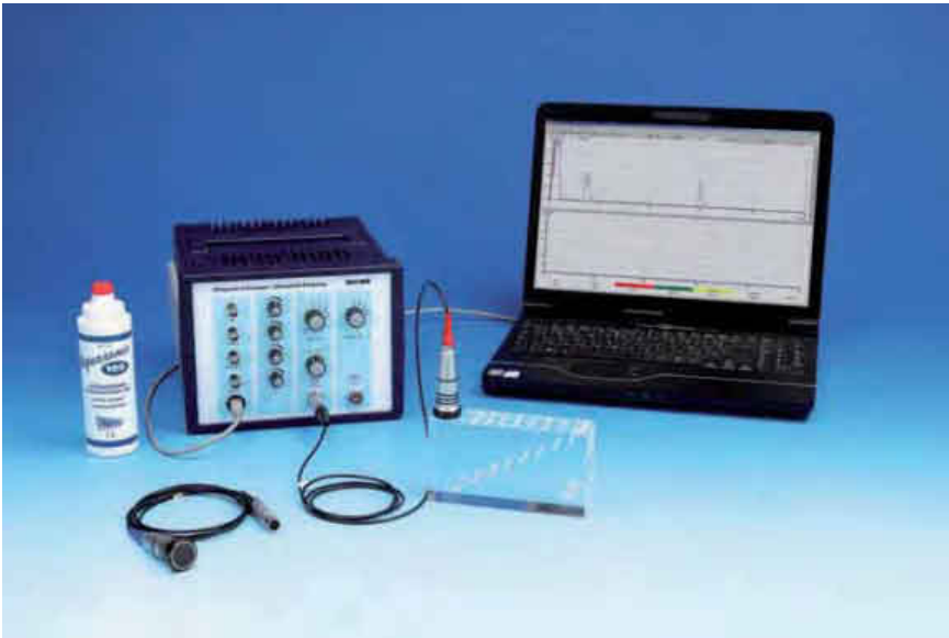
Illustration of the ultraechos, reflected at the two holes, close to each other.
