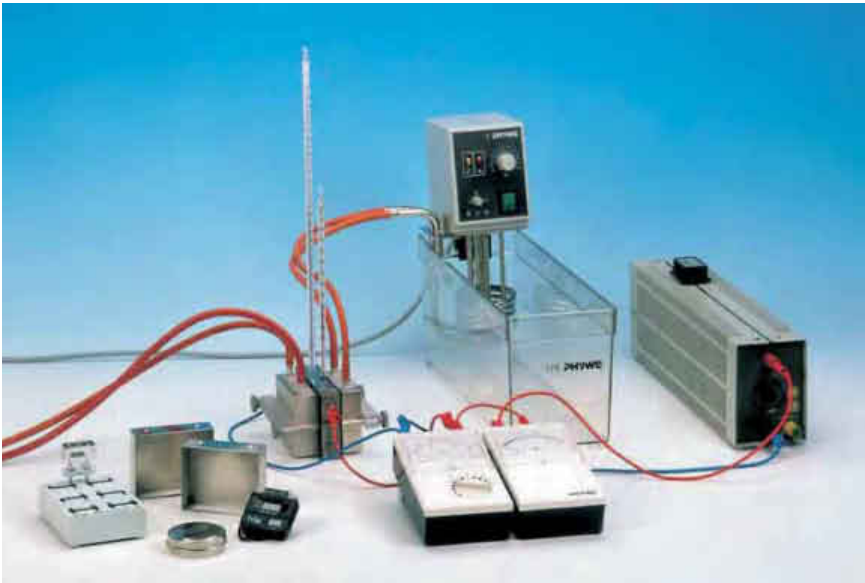
Electrical power generated as a function of the temperature difference.
