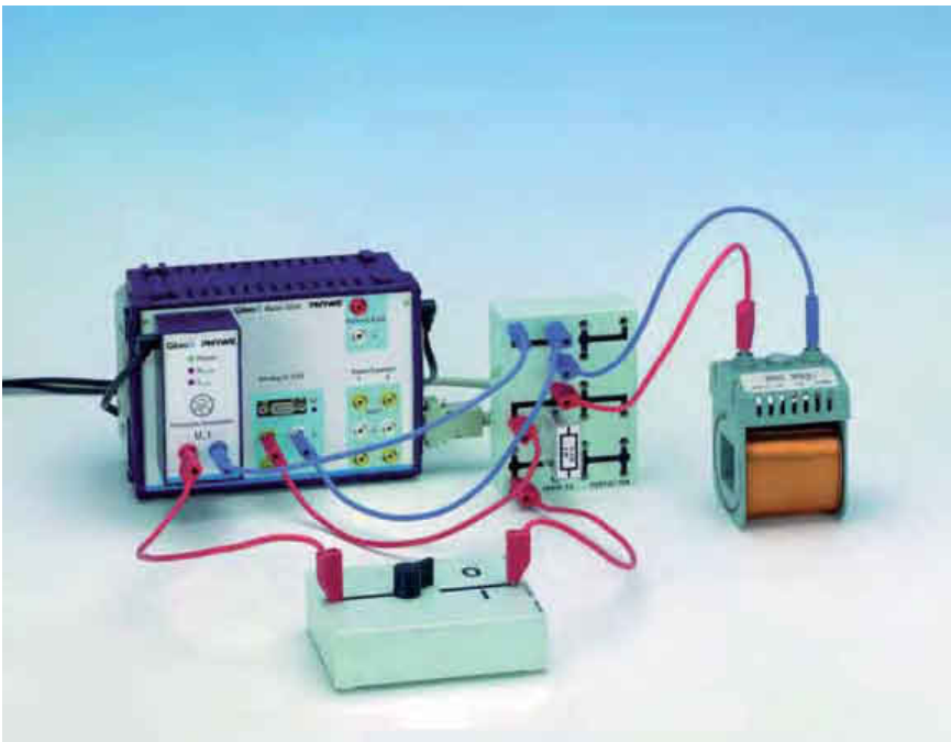
The course of the voltage and the current intensity during a switching on process in a coil.
