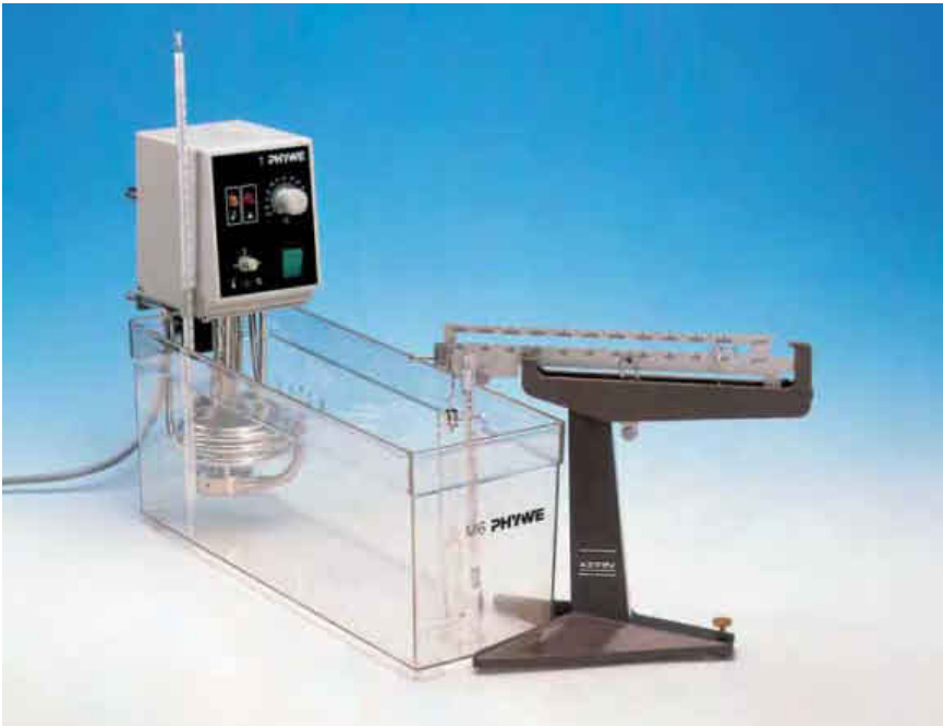
Density of water as a function of temperature.
