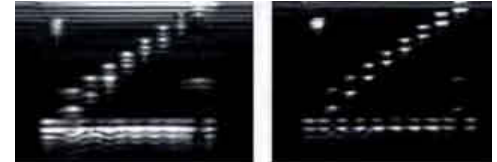
Comparison of the B-scan of the test block measured with a 1 MHz transducer (left) and then with a 2 MHz transducer (right).
