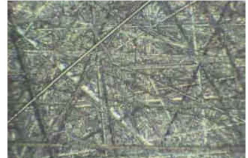
Surface condition of brass sample after step 1 (MD-Primo 220; Lubricant: water; Time: 2 min; Speed: 300 rpm): Magnification: 100x.
