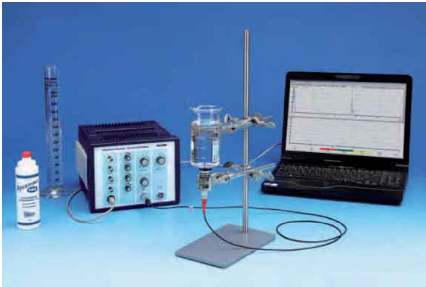
Set-up of the ultrasonic probe for monitoring limit values and for continuous measurements.
