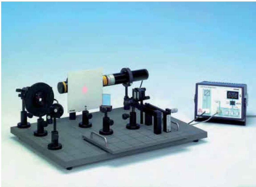
Multibeam interferometer after Fabry and Perot. Illustration of the principle for deriving the individual amplitudes.
