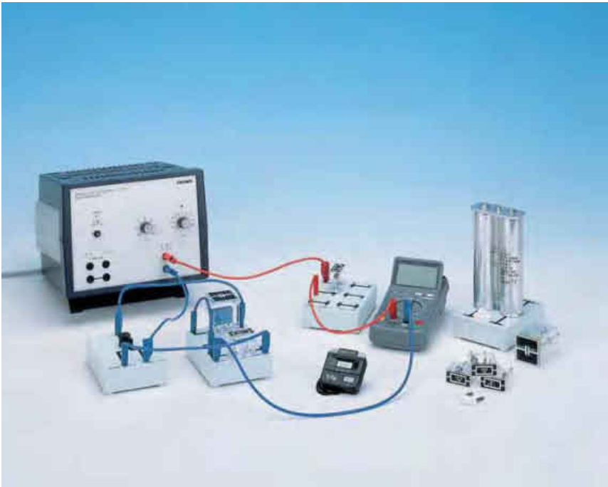
Course of current with time at different capacitance values; voltage and resistance are constant ( U = 9 \text{ V} , R = 2.2 \text{ M} ).
