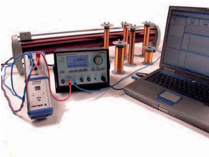
Induced voltage as a function of current for different coils.
