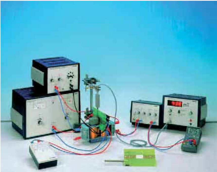
Hall voltage as a function of magnetic induction B , using a copper sample.
