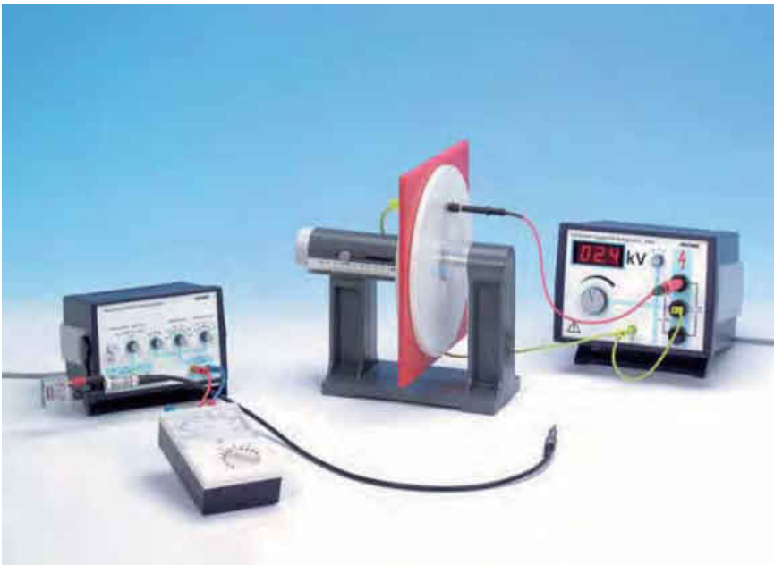
Electrostatic charge Q of a plate capacitor as a function of the applied voltage U_c , with and without dielectric (plastic) between the plates ( d = 0.98 cm).
