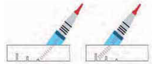
Reflection of an ultrasound beam at a small crack (left) and at a deep crack (right).
