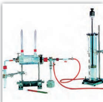
Determination of the heat of formation for CO 2 and CO (Hess' law) (P3021601)
