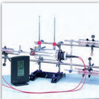
Determination of the heat of formation of water (P3021501)
