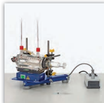
Determination of the molar mass of a liquid (P3010501)
