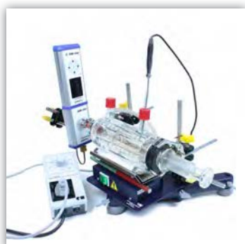
Equation of state for ideal gases with Cobra4 (gas laws: Gay-Lussac, Amontons, Boyle) (P2320162)
