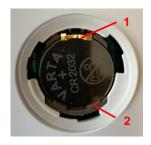
Push the battery into the socket by pressing lightly on the opposite side.
