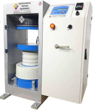
The very silent power pack can load specimens between 1KN/sec to 20KN/sec. On the dual-stage pump, a high delivery low-pressure pump is used for rapid approach and delivery high-pressure radial piston pump is used for test execution. On all power packs, the maximum pressure valve is used to avoid machine overloading.
