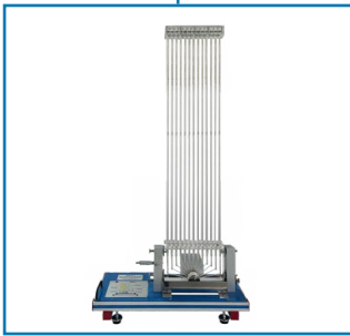
MEMT-1. Radial Pressure Distribution in a Journal Bearing
