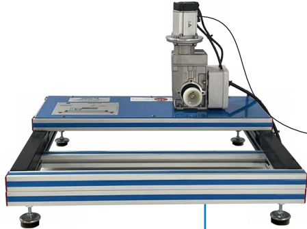
MEMT-UB. Drive Unit for Tribological Tests
