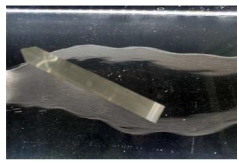
Flow through a flat plate with one triangular end and one rectangular end made of methacrylate.
