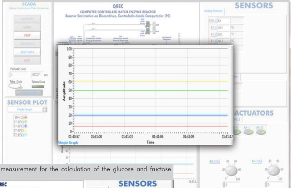
Angle of rotation of the polarized light measurement for the calculation of the glucose and fructose concentration.
