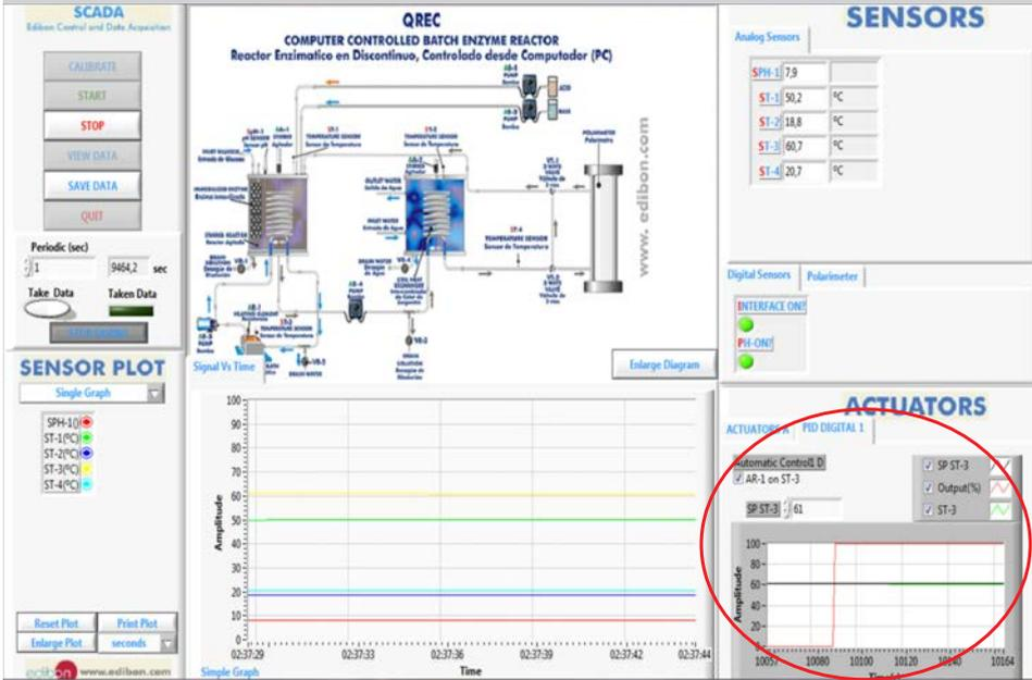
Representation in real time of the measured magnitudes. A single graph showing the temperatures and pH.
