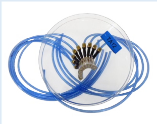
TA12. Concave Semi-Cylinder Model
