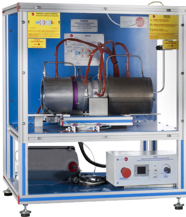
① Unit: TGFAC. Computer Controlled Axial Flow Gas Turbine/ Jet Engine
