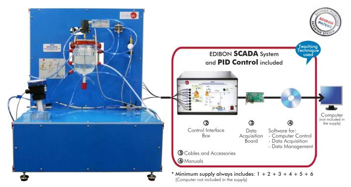
1 Unit: QUCC. Computer Controlled Crystallization Unit
