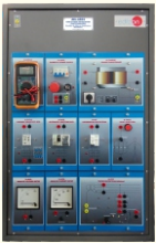
AEL-AD33. Single-Phase Installations Faults Application.
