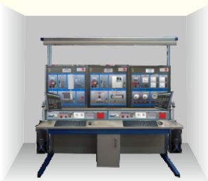
Entry Phone Application and Luminosity Control Workbench
