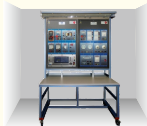
Differential Switches and Luminosity Control Workbench
