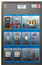
AEL-AD33T. Three-phase Installations Faults Application.
